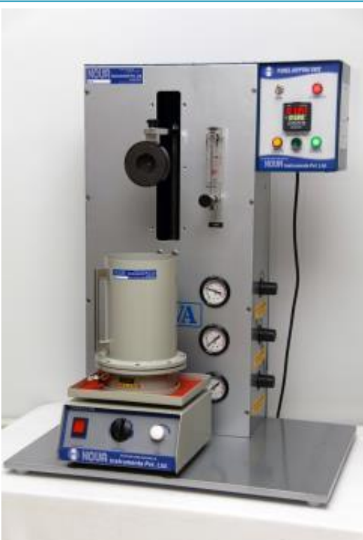
Single Dipping Sample Preparation
